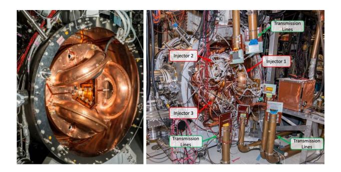
Two photos of the team's prototype reactor, showing the three injectors with (right) and without (left) the electrical circuits (labeled in green on the right) used to form magnetized plasmas in each injector. The GPU precisely controls each of these circuits, allowing the researchers to fine-tune plasma formation in each injector. The individual plasmas then combine and naturally organize into a doughnut-shaped object, similar to a smoke ring. Credit: University of Washington
