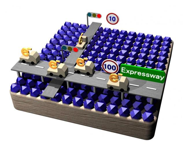
Depending on the orientation of the crystals, the electrical conductivity in the parallel direction in this image is about 10 times higher than that in the vertical direction. Credit: M. Takahashi & K. Okada, Osaka Prefecture University
