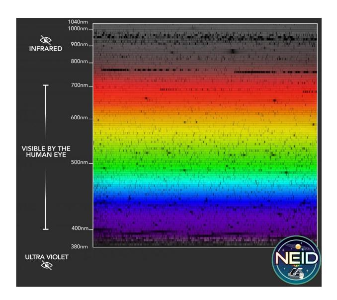
An image of NEID's spectroscopic observations of the Sun. NEID's spectral coverage extends significantly redder and bluer than the limits of human vision, enabling it to observe many critical spectral lines. NEID's design enables high spectral resolution, large wavelength coverage, and exquisite stability. The image
