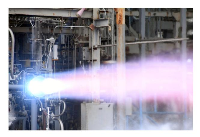
The 3D-printed thrust chamber assembly of the methane-fuelled M10 rocket engine passed its first series of hot firing tests at the NASA Marshall Space Flight Center in the USA during February 2020. The M10 engine will power the upper stage of future Vega evolutions from 2025. Credit: ESA/NASA
