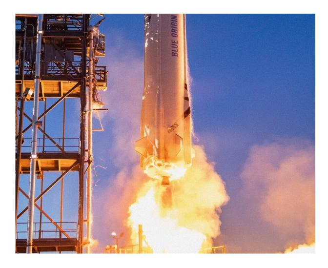
Blue Origin's New Shepard rocket burns liquid hydrogen and liquid oxygen, which combusts as water vapor.
