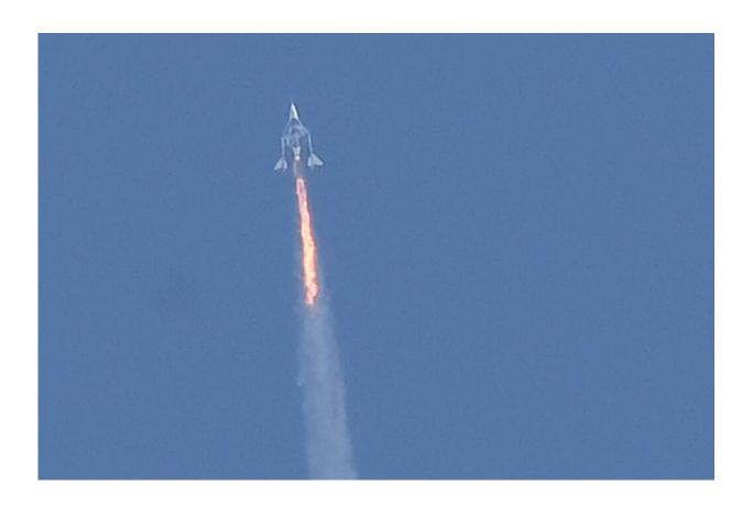
Virgin Galactic's SpaceShipTwo uses a type of synthetic rubber as fuel and burns it in nitrous oxide, a powerful greenhouse gas.
