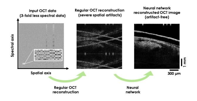
Deep learning improves image reconstruction in optical coherence tomography using significantly less spectral data. Credit: Ozcan Lab @UCLA.
