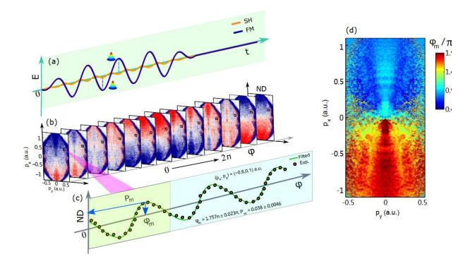
A second harmonic is introduced into a strong fundamental field to disturb the tunneling ionization process. By changing the relative phase of the two-color field, the strong-field tunneling ionization PEMD is perturbed by the SH field. By monitoring and analyzing the relative phase where the photoelectron yield maximizes, researchers can accurately resolve the quantum orbits at each momentum. Credit: J. Tan, et al
