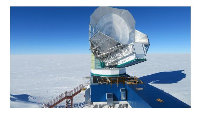
The South Pole Telescope is part of a collaboration between Argonne and a number of national labs and universities to measure the CMB, considered the oldest light in the universe. The high altitude and extremely dry conditions of the South Pole keep water vapor from absorbing select light wavelengths. Credit: Argonne National Laboratory.
