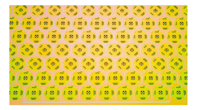
A section of a detector array with architecture suitable for future CMB experiments, such as the upcoming CMB-S4 project. Fabricated at Argonne's Center for Nanoscale Materials, 16,000 of these detectors currently drive measurements collected from the South Pole Telescope. Credit: Argonne National Laboratory
