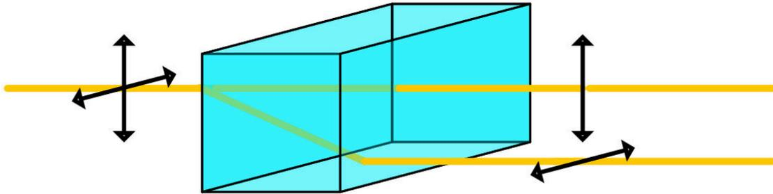
Bending polarized light: This illustration shows how light with different polarization directions (indicated by black arrows) passes through a material along two different paths (yellow beams). This is called the birefringence effect. Results from RHIC provide evidence that birefringence also happens in a magnetic field in a vacuum. Credit: Brookhaven National Laboratory
