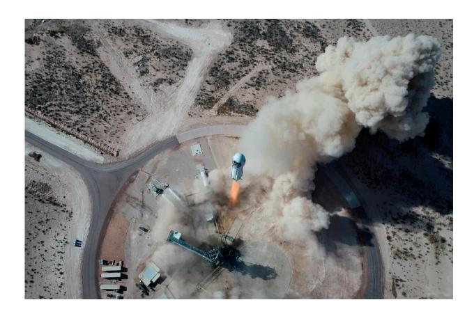
In this Jan. 14, 2021 photo made available by Blue Origin, the New Shepard NS-14 rocket lifts off from Launch Site One in West Texas. On Tuesday, July 20, 2021, Blue Origin's 60-foot (18-meter) New Shepard rocket will accelerate toward space at three times the speed of sound, or Mach 3, before separating from the capsule and returning for an upright landing. Credit: Blue Origin via AP
