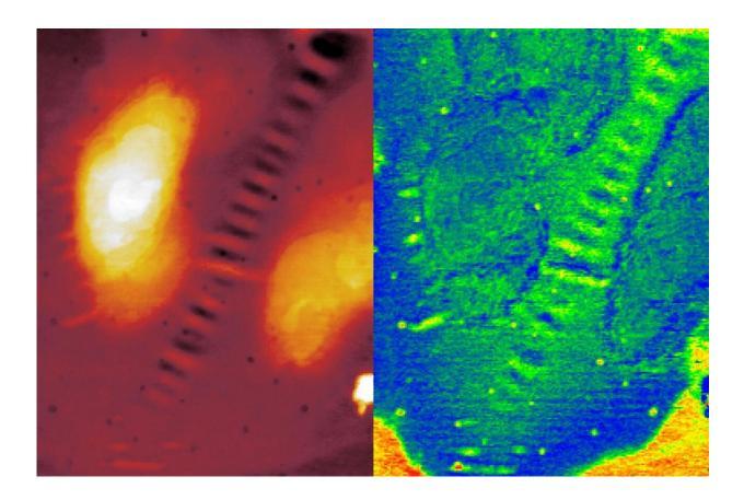
Bitumen surface imaged with different microscopic techniques: AFM (topography image) and AFM-IR (chemical distribution - IR absorption at 1262 cm-1). Credit: TU Wien
