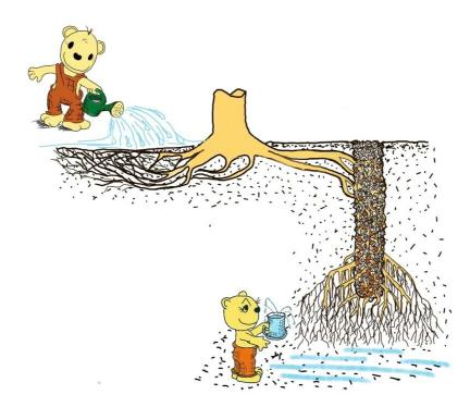
The gravel cylinder method could also draw tree roots into deeper soil layers. This can help the tree to deal with increased drought. Credit: Claus Mattheck, KIT
