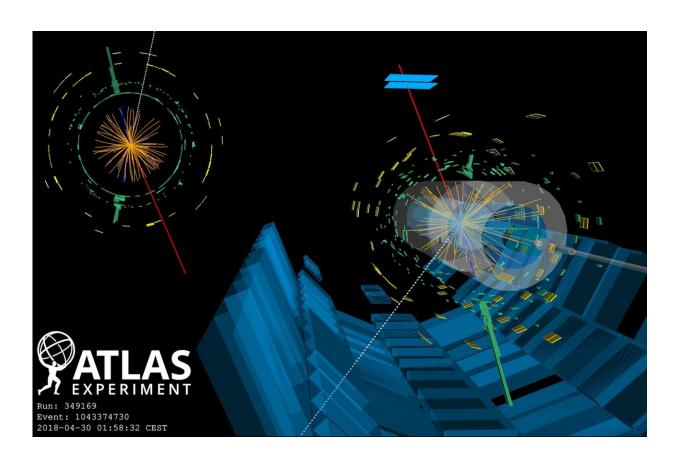
Display of a candidate WWW→ 3 leptons + neutrinos event. The event is identified by its decay to a muon (red line), two electrons (blue lines), and missing transverse energy (white dashed line). Credit: ATLAS Collaboration/CERN
