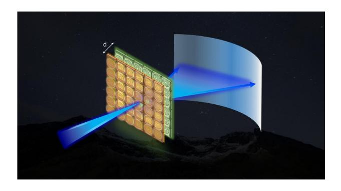
Illustration of a planar telescope consisting of two layers of flat optics for achieving angle magnification. Both layers are assigned phase profiles following the sum of even order polynomials and they are separated in space by d. Credit: Ziqian He, Kun Yin, and Shin-Tson Wu
