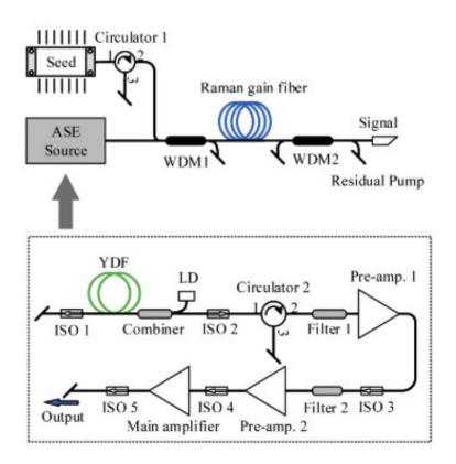
Fig. Schematic of the single-frequency RFA in co-pumping configuration. Credit: SIOM
