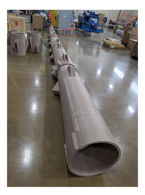
ORNL researchers demonstrated a 3D-printed power pole made of bioderived
