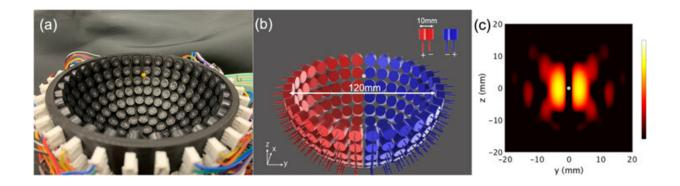
Fig. 1. (Color online) (a) Levitation by hemispherical transducer arrays (b) mounting of transducers on the array of diameter is 120 mm. (c) Distribution of the relative acoustic pressure on the vertical cross-section calculated by numerical simulation based on geometrical acoustics when capturing a particle at the center of the hemispherical array (the origin). Credit: Tokyo Metropolitan University
