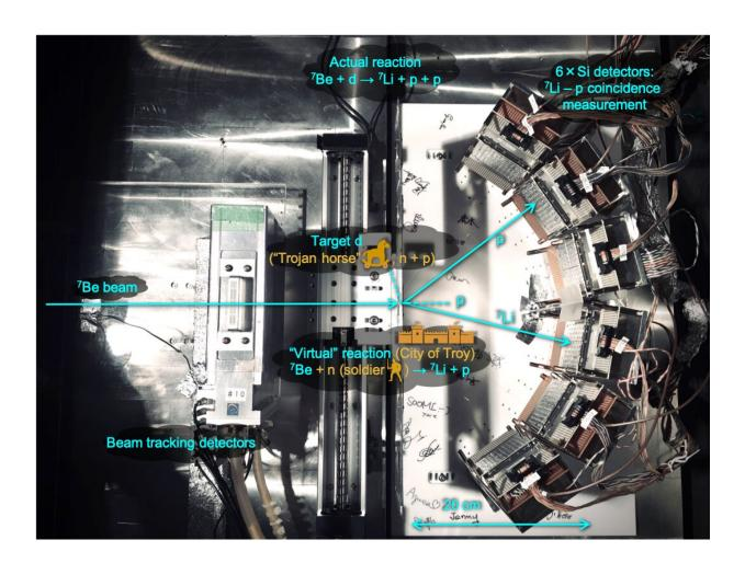
Experimental setup. As a beam of beryllium comes in from the left, the deuteron Trojan horse intercepts it at the target and delivers its neutron soldier. This allows the decay products of the beryllium and neutron reactions to be captured by a curved array of six detectors on the right. Credit: Hayakawa et al.
