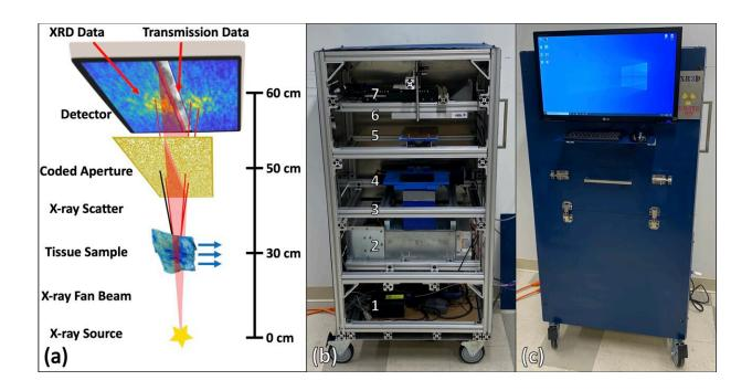
This prototype x-ray scanner produces images complete with internal molecular composition with unprecedented resolution and accuracy by analyzing how x-ray bounce off of the samples. Credit: Joel Greenberg, Duke University
