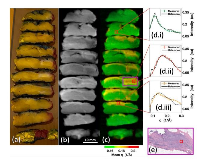
The new x-ray scanner can detect cancerous tissue within biopsies, potentially helping surgeons to ensure all cancerous tissue is removed or providing a new method for making diagnoses. Credit: Joel Greenberg, Duke University
