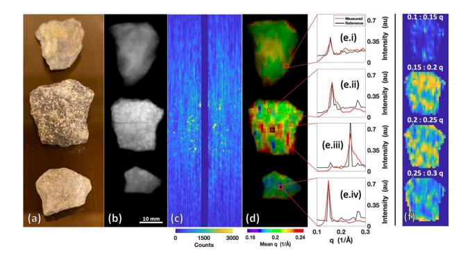
The new x-ray scanner can provide detailed information about the internal makeup of rocks, which could be useful for archaeologists studying fossils or miners making decisions about which ore to use in their extraction facilities. Credit: Joel Greenberg, Duke University
