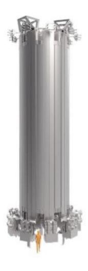
The Central Solenoid, the largest of ITER's magnets, will be made up of six modules. It is one of the largest of the U.S. contributions to ITER. Credit: ITER / General Atomics
