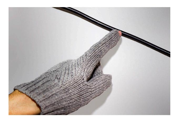
The fingertips of a wireless voltage detection glove illuminates when the wearer's hand approaches a live cable. Credit: Purdue University/Rebecca McElhoe
