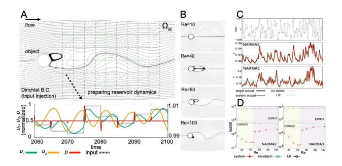
A: Outline of the study. B: Typical fluid flow at each Reynolds number. C: Inputs along time sequence and the results of NARMA2 and NARMA3 models. Target values are in black while values by virtual physical reservoir computing using vortices are in red. D: Values of errors (normalized mean square errors, NMSE) at each Reynolds number in NARMA2 and NARMA3 models. The error is minimal with Reynolds number being around 40. Credit: Kanazawa University
