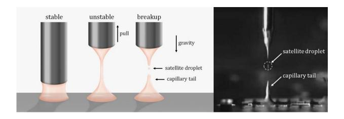
The conventional method of breaking liquid bridges uses retraction. When the nozzle (or plate) is lifted, the liquid bridge extends and breaks. This can form capillary tails and satellite droplets. Researchers in the OIST Micro/Bio/Nanofluidics Unit are studying cleaner methods of breaking liquid bridges, and have reported their results in a PNAS study. Credit: OIST
