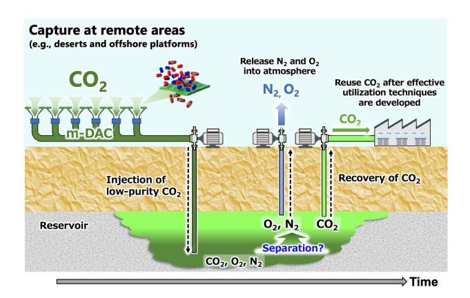
Schematic image of low-purity CO2 storage with the membrane-based Direct Air Capture (DAC). Credit: Takeshi Tsuji
