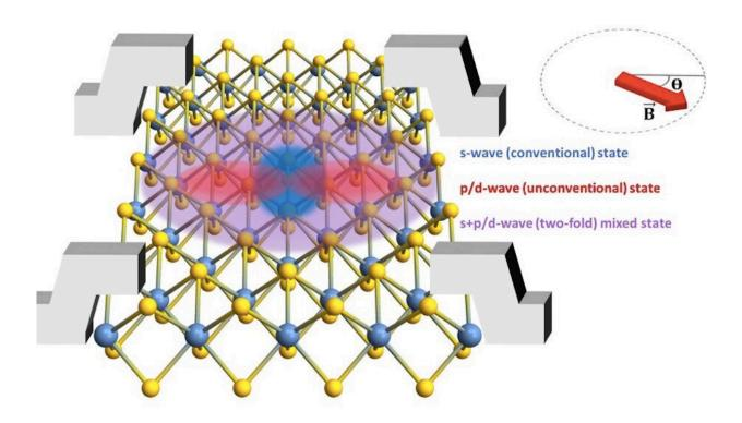
A team of physicists led by the University of Minnesota has discovered that the unique superconducting metal Niobium diselenide (NbSe2) is more resilient when used as a very thin layer. The above diagram depicts the different s-, p-, and d-wave superconducting states in the metal. Credit: Alex Hamill and Brett Heischmidt, University of Minnesota
