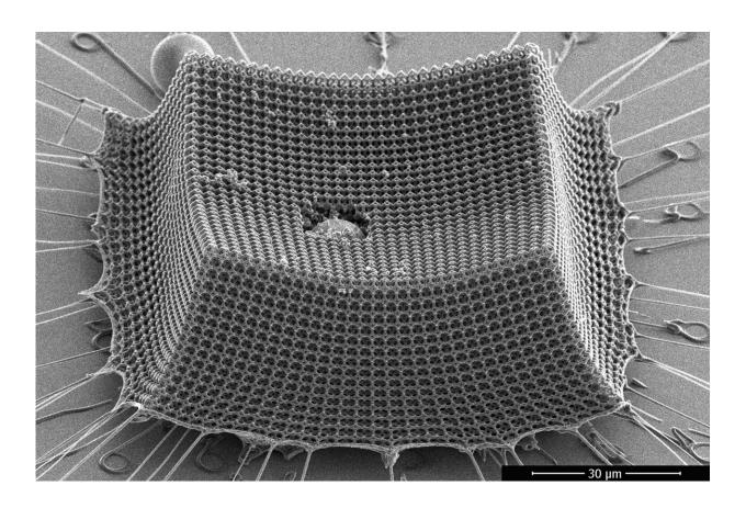
Engineers at MIT, Caltech, and ETH Zürich find "nanoarchitected" materials designed from precisely patterned nanoscale structures (pictured) may be a promising route to lightweight armor, protective coatings, blast shields, and other impact-resistant materials. Credit: Carlos Portela et al
