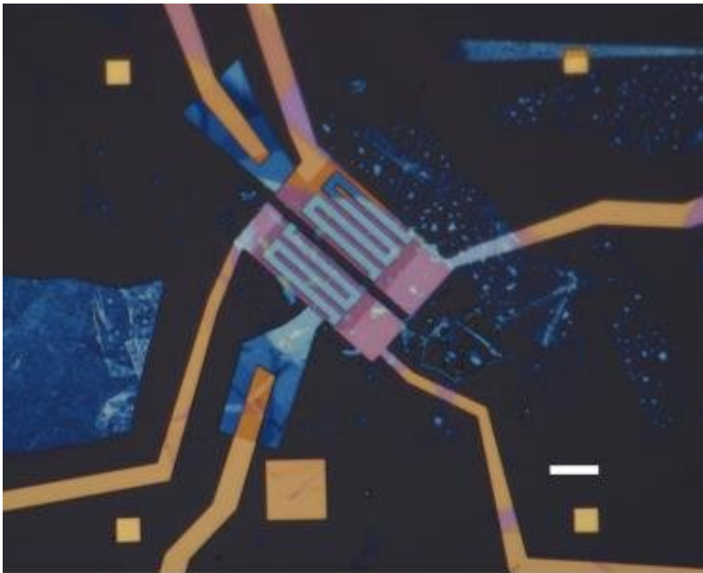
An optical micrograph of two typical on-chip spectrometers. Scale bar: 8 micrometers
