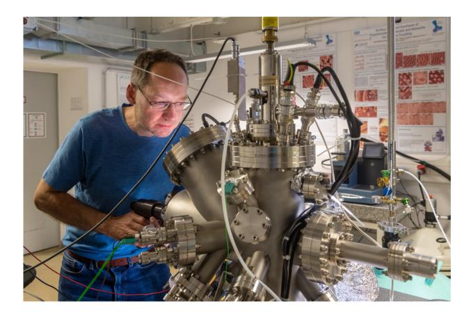
Markus Lackinger transferring a sample inside the ultra-high vacuum chamber by means of a vacuum grabber. This vacuum chamber contains all facilities for preparing and analyzing samples in vacuum. Credit: Andreas Heddergott / TUM
