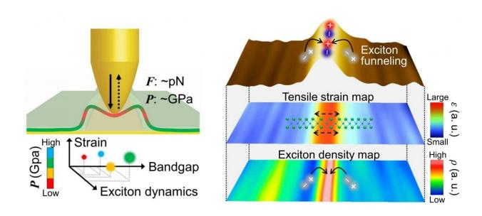
Schematic diagram of a-TEPL spectroscopy based on shear-force AFM using bottom-illumination optics with a 632.8 nm He/Ne laser. Credit: UNIST
