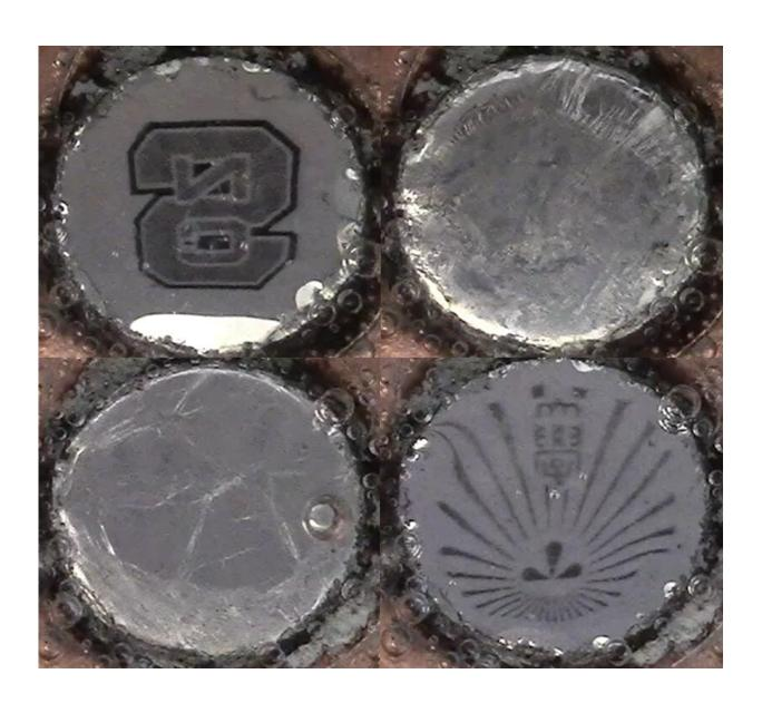
Researchers have developed a way to dynamically switch the surface of liquidmetal between reflective (top left and bottom right) and scattering states
