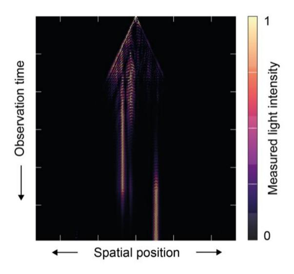
The figure shows the experimentally measured light propagation: Initially diverging light is intermittently focused into a tiny spatial region by disorder. After some time, the signal suddenly appears at an entirely different position, seemingly without having to traverse the intervening medium. Credit S. Weidemann, M. Kremer et al.
