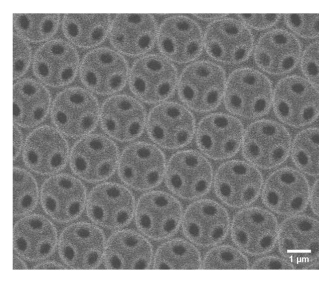
A representative scanning electron microscopy image of inverse opals, the porous medium used in this research. Large circular patterns indicate the close packed cavities, and small elliptical patterns indicate the holes connecting adjacent cavities. Every cavity was connected to its adjacent cavities through twelve holes. Credit: Haichao Wu
