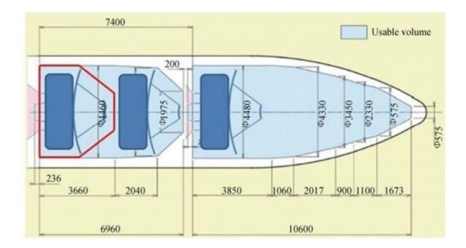
Mode of how the EHI could fit in to an Arianne 6 rocket, with room to spare. Credit: Kudriashov et al.
