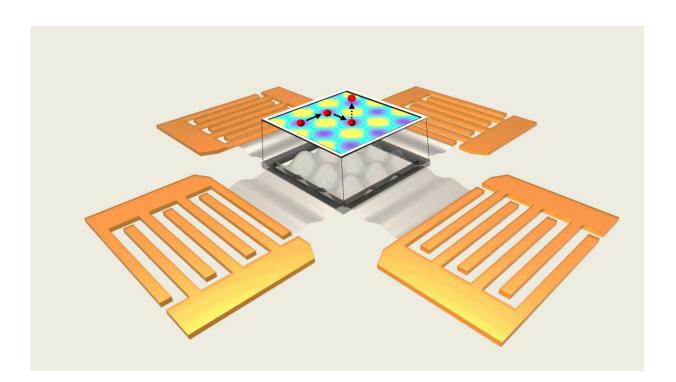
This new biomedical device manipulates particles as small as DNA (2.5 nanometers) with sound-induced electric fields. Four transducers send sound waves into a substrate that creates electricity as it vibrates, producing patterns of electric-acoustic waves that control particles in the liquid-filled chamber above. Credit: Peiran Zhang, Duke University
