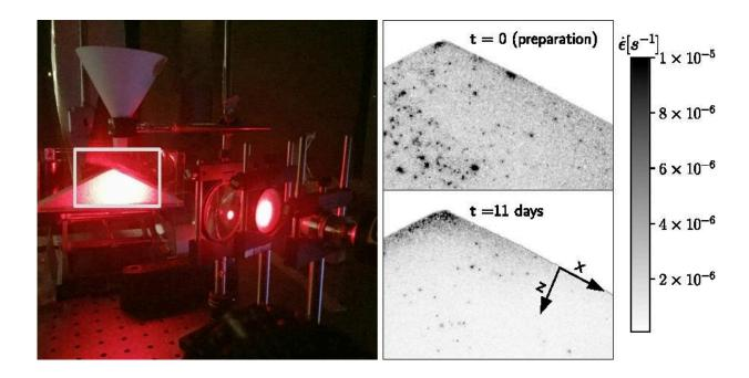
In the Jerolmack lab, diffusion-wave spectroscopy was used to study very small grain movements in piles of sand (shown in panel on the left). The data that was collected, depicted in strain rate maps (in panel on the right), shows that grain activity continues after 11 days without disturbance. Credit: Nakul Deshpande
