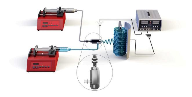
Schematic of co-axial electrospinning device. Credit: Elsevier
