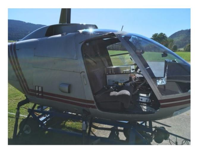
The spectropolarimeter instrument FlyPol aboard the helicopter, with which the team carried out the experiment. Image Credit: Jonas Kühn
