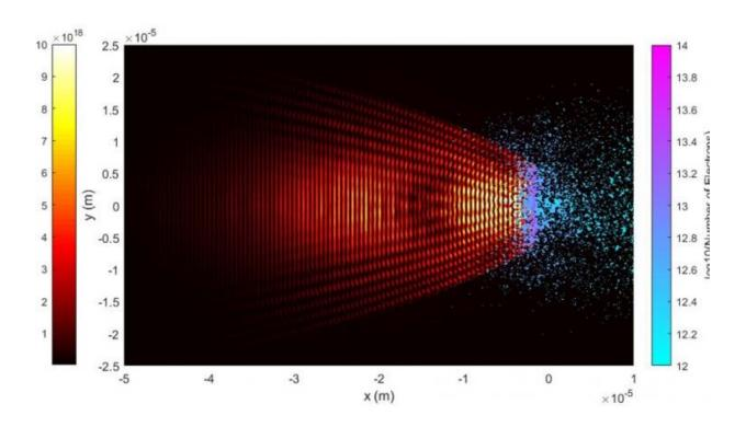
This image shows the intensification of the laser in simulations and the electrons being accelerated. Credit: Lawrence Livermore National Laboratory
