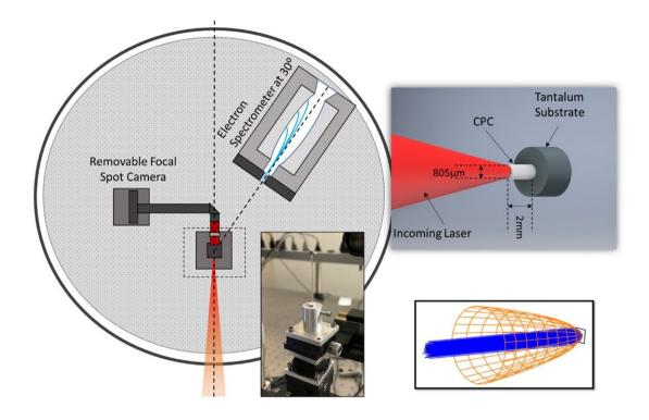
This image shows the experimental setup displaying the target, laser and electron spectrometer. A 3D drawing of the CPC, tantalum substrate and the incoming laser also is shown. Credit: Lawrence Livermore National Laboratory
