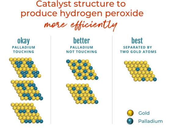
University of Illinois researchers demonstrate a more efficient and environmentally friendly method to produce hydrogen peroxide with palladium-gold nanoparticles, a catalyst that they found performs better when the palladium particles are surrounded by gold. Credit: Claire Benjamin/University of Illinois
