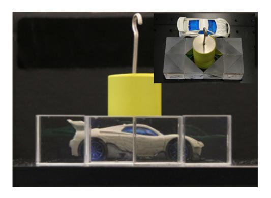
Cloaking device realized by standard optical components. Credit: Figure reproduced with permission from Sci. Rep. 6, 38965 (2016) Copyright 2016 Springer Nature Limited
