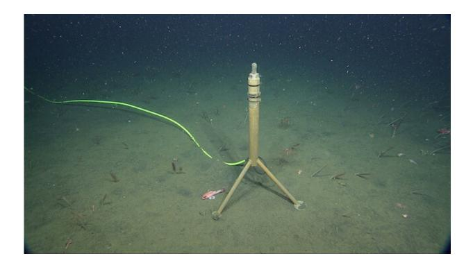
The hydrophone at MBARI's MARS ocean observatory has been instrumental for observing the soundscape of Monterey Bay and beyond. A cable runs from the instrument to the observatory and back to shore, providing power and a high-
