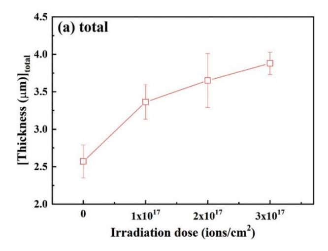
Fig. 3. Variation of oxide film thickness of T91 steel with irradiation dose (450 °C, 5 m/s, 10 MPa, 5 ppb). Credit: LIU Chao
