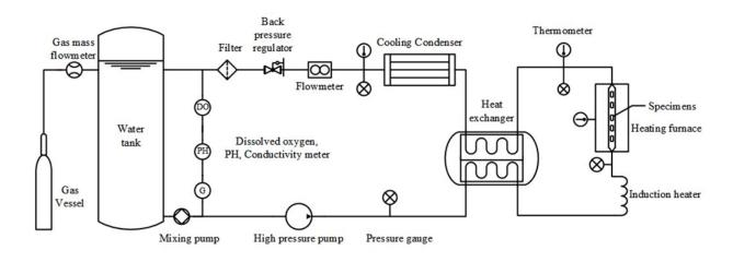
Fig. 1. Schematic diagram of the high temperature and high pressure water dynamic corrosion device. Credit: LIU Chao
