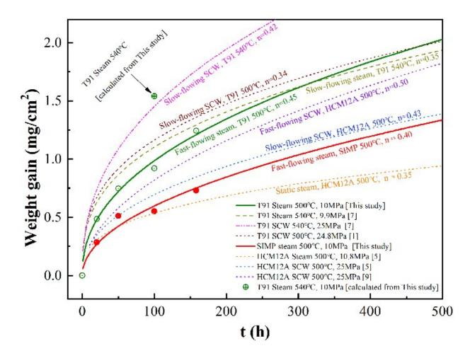
Fig. 2. Corrosion kinetics curves of SIMP and T91 steels (5 m/s, 5 ppb). Credit: LIU Chao
