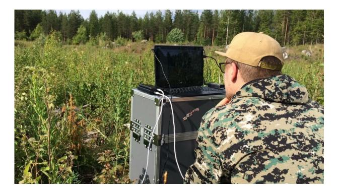
Air traffic control station in a felling site. Researcher Anton Kuzmin is monitoring the progress of a fixed wing drone flight. Credit: University of Eastern Finland
