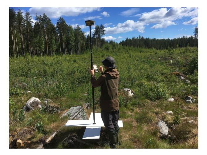
Marking aerial imaging correction points with a GPS device. Credit: University of Eastern Finland
