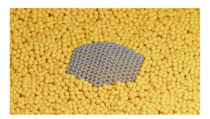
Snapshot from MD simulation of graphene on liquid Cu. Credit: Santiago Cingolani
