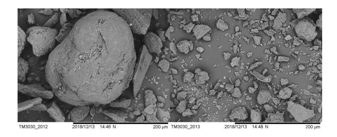
In the control image (left), the substrate is smooth and intact, but in the image following NaOH-urea pretreatment (right), the substrate is broken down. Credit: Harbin Engineering University
