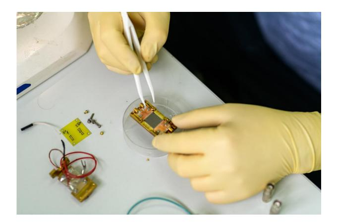
Mounting a superconducting chip on a board. Credit: Andrey Zmeev, MIPT Press Office
