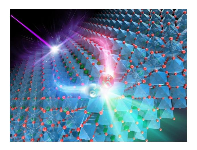
Charge recombination occurs when mobile charge carriers present in the material that are exposed to light annihilate each other and can hamper the energy efficiency of the photocatalyst. Credit: Masashi Kato from Nagoya Institute of Technology
