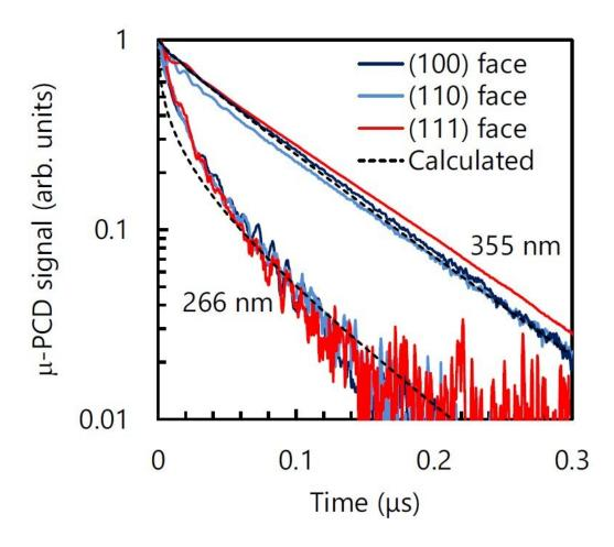
The figure shows  $\mu$ -PCD decay curves for the undoped samples excited by the 266- or 355-nm laser. The dotted line is the calculated decay curve with  $\tau B = 90$  ns and S = 106 cm/s. Credit: Masashi Kato from Nagoya Institute of Technology
