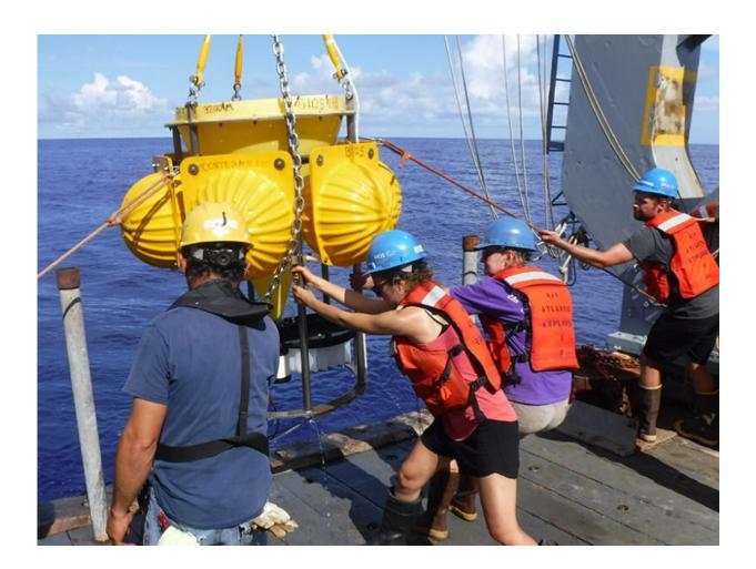
An Oceanic Flux Program time series sediment trap deployed at 3,200-meter depth comes on board the R/V Atlantic Explorer. Credit: J. C. Weber
