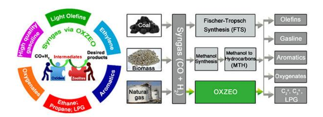
Oxide-zeolite-based composite catalyst concept that enables syngas chemistry beyond Fischer–Tropsch synthesis. Credit: JIAO Feng and MIAO Dengyun
