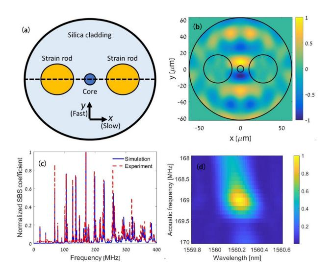
a, Schematic cross-section of a "panda-type" fiber. Two strain rods induce strain in the fiber, and distinguish between propagation in "slow" and "fast" axes. b, Profile of material displacement of an acoustic wave supported by the panda fiber cross-section. c, Measurement and calculations of the spectrum of acoustic waves that are driven by light in the panda fiber. The acoustic waves are stimulated by a pair of optical tones: one polarized along the fast axis and the
